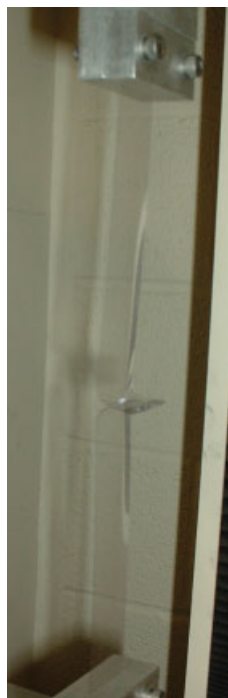
FIG. 4. A sample mounted in a T -peel arrangement in the custom grips. This test is designed to measure the force required to peel apart the spot welded samples. [Color figure can be viewed in the online issue, which is available at www.interscience.wiley.com .]
